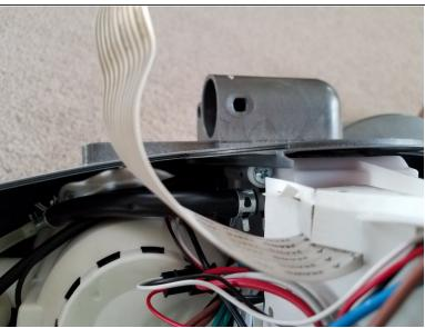
Remove the two screws and gently move white box with wires out of the way.
