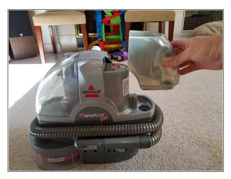
Remove cleaning solution tank.
