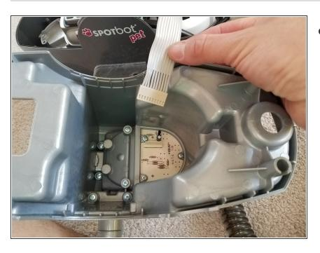
Remove top cover. Unplug ribbon cable from control board and set top aside.
