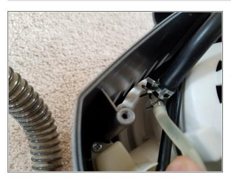
Locate end of clear rubber tubing and remove clamp with pliers. It is nearly impossible to get the hose end off of the hose barb, so I just cut the hose close to the barb, then gently scored the tubing left on the barb to get it off.
