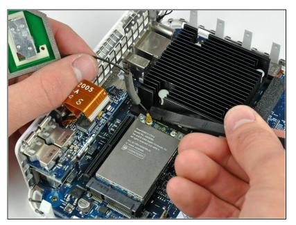
Use the flat end of a spudger to pry the AirPort antenna cable connector up off the AirPort card.
