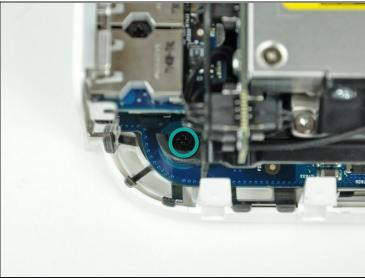
• Remove the Phillips screw near the audio ports securing the internal frame to the bottom case.
