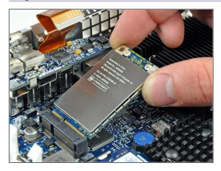
Lift the AirPort card up slightly and pull it away from its socket on the logic board.
