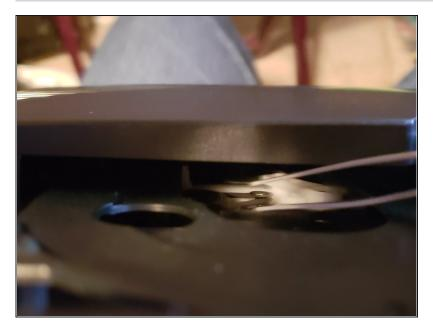
• There will be a gap in the middle of the CD/DVD tray. You will see 2 pulleys with a rubber belt. Use <u>tweezers</u> to carefully take the belt out.
