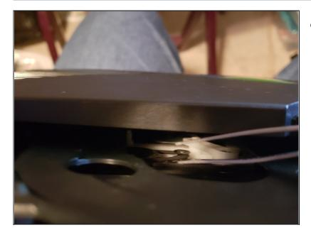
• Using the tweezers again carefully put the rubber belt back in. I have found it easier to get it around the big pulley first then on the small pulley.
