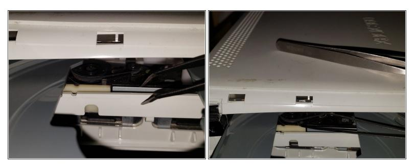
Use tweezers to take a rubber belt of 2 pulleys in between the hole in the DVD Tray.
