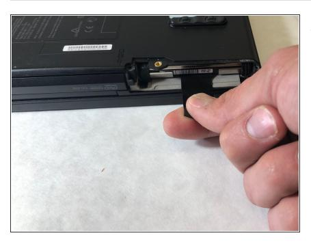
Use the pull tab on the hard drive to completely pull out the hard drive.
