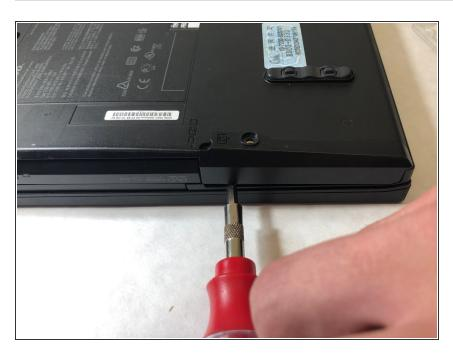
Use a flathead screwdriver to gently pry up the cover and remove it completely.
