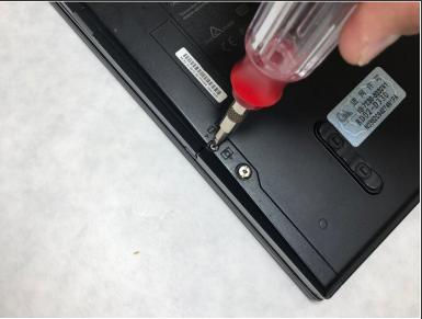
Using a flathead screwdriver, remove the two screws that are holding the hard drive cover in place on the back corner of the computer.
