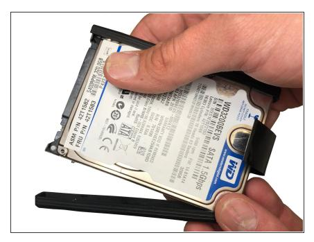
Remove the side bumpers from the original hard drive and place them on the new hard drive.
