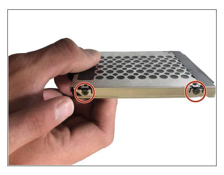
Using a #00 Phillips head screwdriver, remove all four screws on the hard drive cover.
