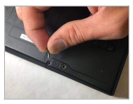
Put cover back on computer and tighten screws with a flathead screw driver.
