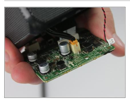
You can then remove the speaker cable and the top board cable. To reassemble your device, follow these instructions in reverse order.
