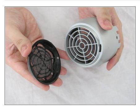
Remove the black vent from the grey cylindrical piece.
