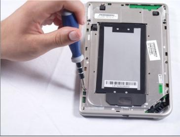
• Using the T5 Torx screwdriver, remove the ten T5 screws from around the edges of the silver midframe.
