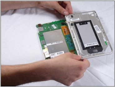
• Carefully lift the silver midframe away from the motherboard and display assembly.
