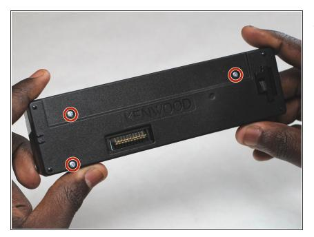
Remove the three 7.5mm Phillips #1 screws.
