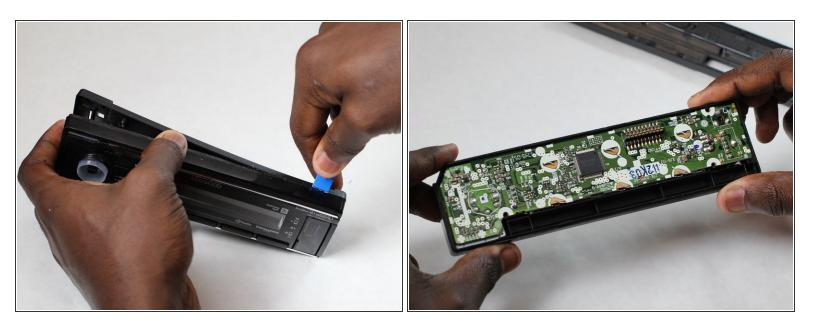
Separate the two halves of the housing by prying along the length of the device with a plastic opening tool.
