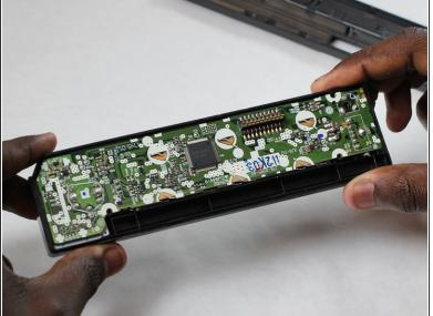
Separate the two halves of the housing by prying along the length of the device with a plastic opening tool.
