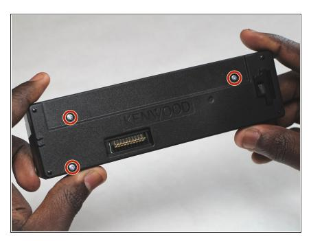
Remove the three 7.5mm Phillips #1 screws.
