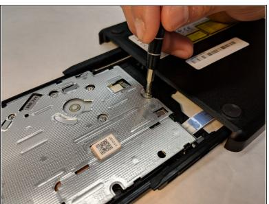
Turn the unit over and remove the two silver 3mm Phillips #0 screws from the aluminum cover.
