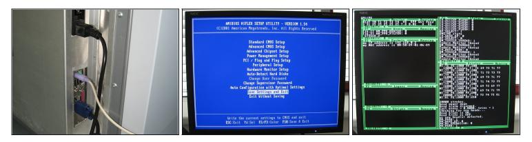
• Before connecting the Ethernet cable, test if the new mainboard has resolved the issue that caused the fault.
