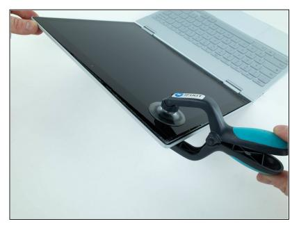
Use an iSclack, or suction cup, to lift up the corner of the display from the case.
