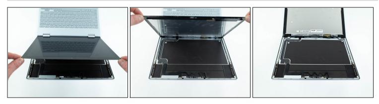
• Flip the display over and lay it flat on the keyboard.
