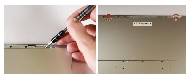
Remove the two yellow 2.0mm screws by using a T3 Torx screwdriver.
