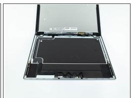
Flip the display over and lay it flat on the keyboard.
