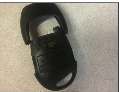
Insert a flathead screwdriver or other small flat tool into the small recess on the back of the to pry
