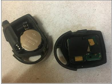
With the bottom section you have now, open it. No tool is needed, just pull the two parts apart which are hinged like a door. (I.e. separate one side first, followed by the opposite side.)
