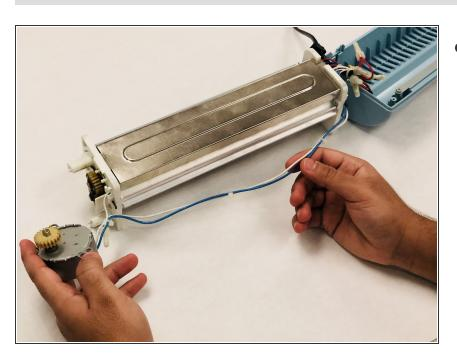
Lift the motor out of the plastic casing.
