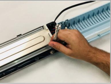
Using the Phillips #2 screwdriver, remove three 8.5 mm long screws and washers on the front edge of the plastic casing.
