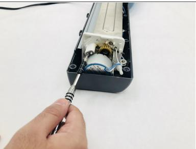
Using the Phillips #2 screwdriver, remove two 9 mm long screws on the side of the main component that keep the motor in place.
