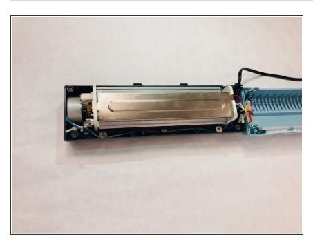
Open the top of the device, and the inside of the Laminator will be exposed as shown.
