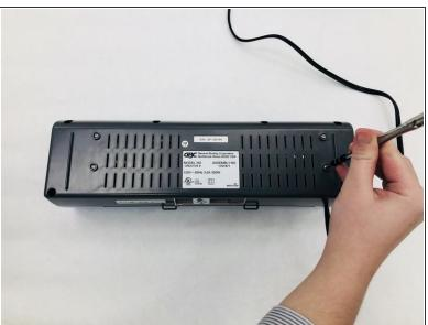
Using the Phillips #2 screwdriver, remove ten 12 mm long screws on the bottom of the device.
