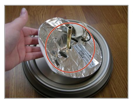
Lift the heat cover, also known as foil, out of the way.
