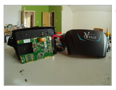
Unplug cables and remove motherboard by uncliping 4 brackets in corners
