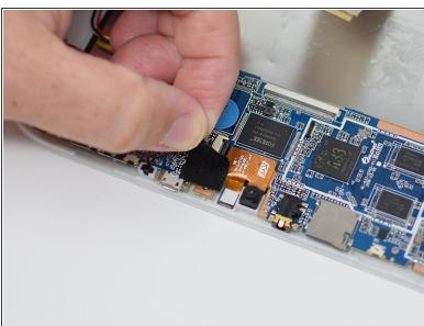
Remove the black tape to reveal the wire ribbon connector.
