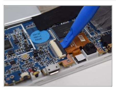
Use the plastic opening tool to flip up the black retaining tab.
