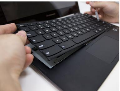
Use the hook of the metal spudger to carefully lift up the keyboard.
