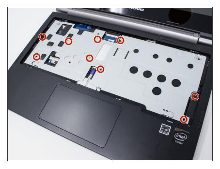
Remove all nine 3.5 mm Phillips #00 screws using a screwdriver.
