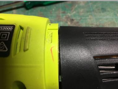
Remove black plastic nose cowling by twisting anti-clockwise
