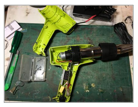
Remove top half housings leaving subassemblies and parts on lower housing
