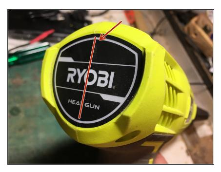
With a sharp blade cut the adhesive label inline with the split line of where the outer housings meet.
