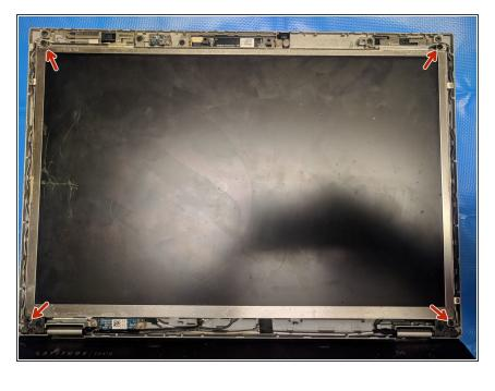
Remove the **four** Phillips #0 screws in the four corners of the display bracket.
