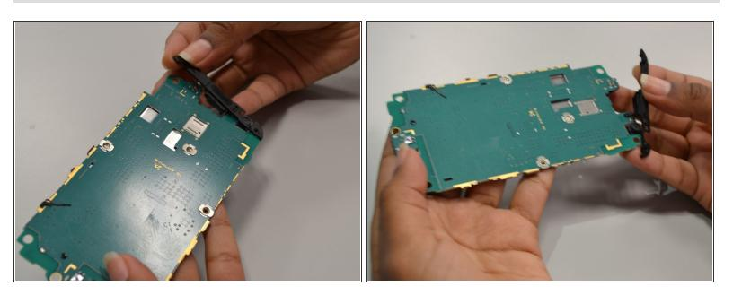
Gently pull the black piece that is connected to the top of the motherboard. This is the speaker.
