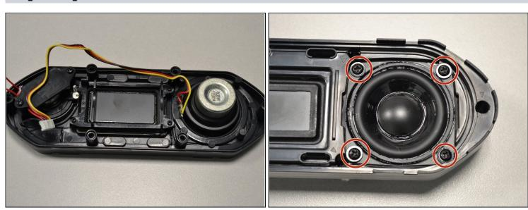
Unscrew the four screws holding the speaker in place.
