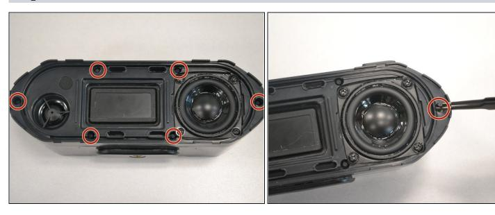
• Use the <u>tweezers</u> to remove the six rubber stoppers. There are four in the middle and two on the sides.
