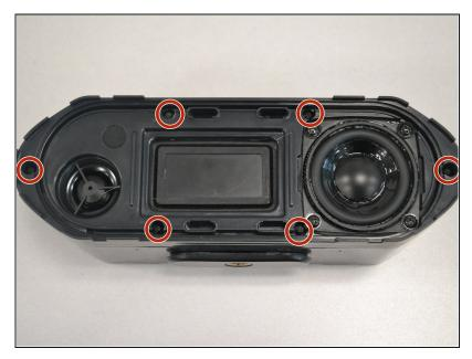
Use the PH1 Phillips screwdriver to remove the six 12mm screws that lie underneath each rubber stopper.
