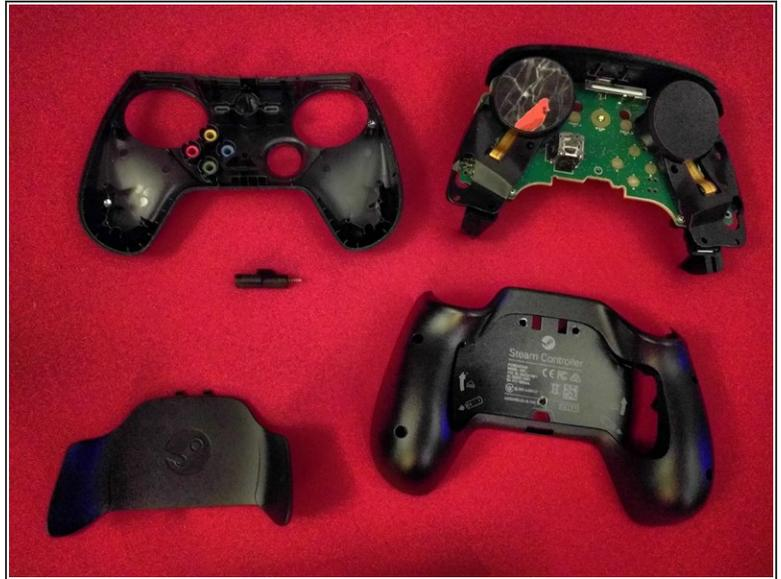
**i** I did not have a long enough screwdriver, so I ended up drilling out two of the four side screws.
