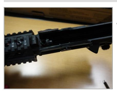
Slide the barrel into the upper receiver.
