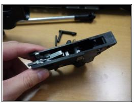
• Insert the selector drum and rotate the leg from the trigger spring downwards so that it locks in the underside of the selector drum.
