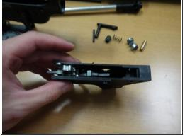
Insert the disconnector spring in round slot on the trigger. Put the disconnector back in the trigger and insert the brass trigger pin through the trigger and the disconnector.
