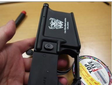
Slide the mag catch spring over the shaft and reinstall the button.
