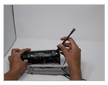
Insert the new button from the inside of the device, pushing it gently towards the front until it locks into place.
