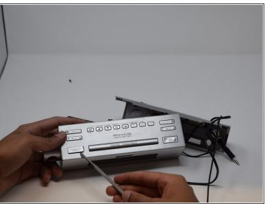
Gently insert a flat head screwdriver in the gaps between the button and device body to loosen them from their positions.
