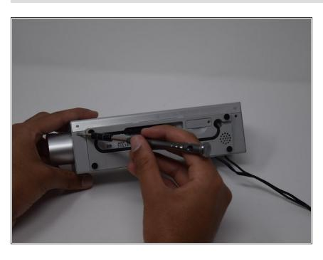
Remove all screws on the back cover of the device and pull the cover off.
