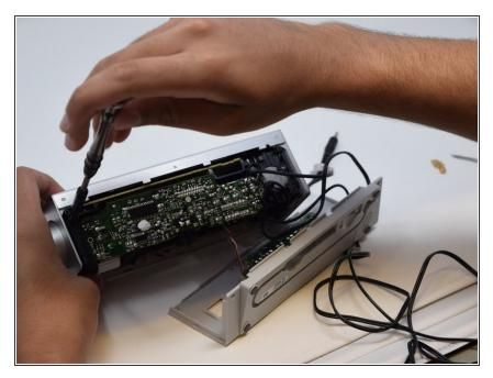
Using a small tool, firmly press on each button until they pop out of their place.
