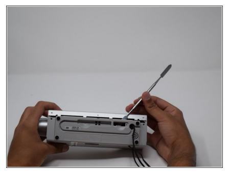
Continue by removing the back cover of the device, pry open with a screwdriver if necessary.
