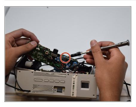
Ensure the batteries next to the antenna have not fried or been damaged.
