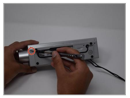
Remove the screw from the backside cover of the Sony Dream Machine with a Phillips Screwdriver.
