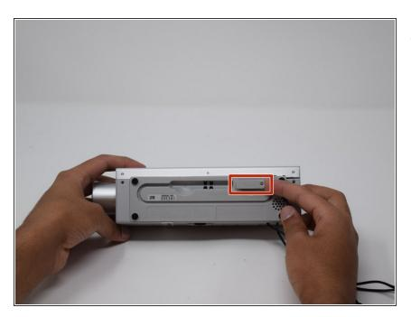
• Using your finger, carefully pull the battery from cover tab.
