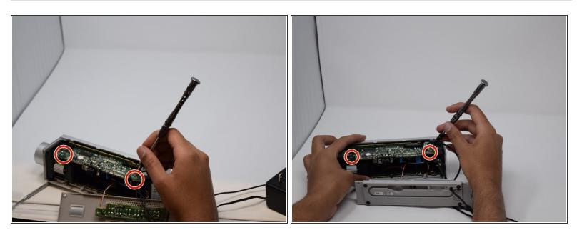
Using a small Philips screwdriver, remove all of the tiny screws from the motherboard.
