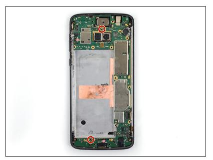
Use a Phillips #000 driver to remove two 2.5 mm-long screws securing the motherboard.
