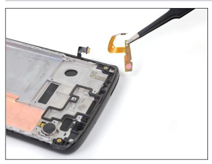
• Remove the front-facing sensor array.
