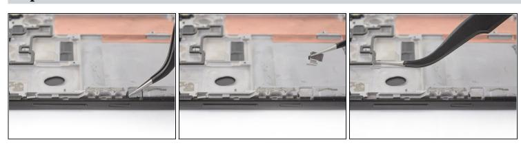
• Use tweezers to lift the two silver retention brackets flanking either end of the volume and power buttons straight up and remove them from the phone.
