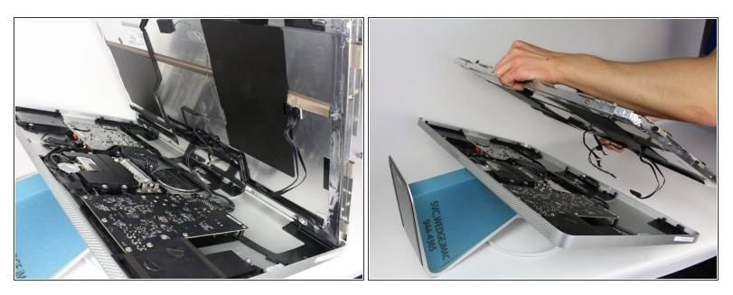
• The LCD has now been fully disconnected from the casing and can be repaired/replaced!
