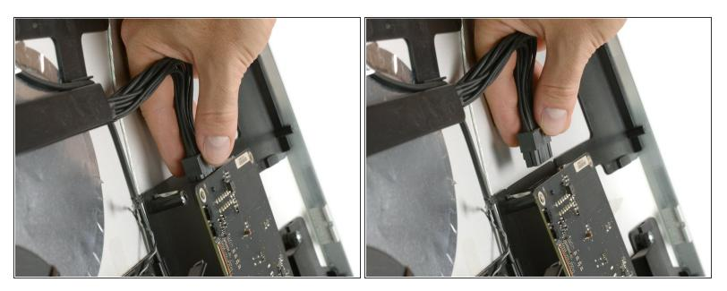
Now you are able to reach behind the logic board to disconnect the cable running to the power board.
