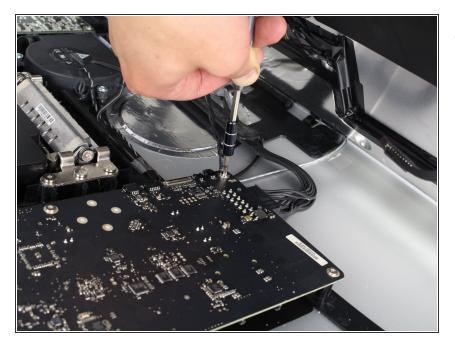
For the last wire connecting to the LCD, use your T 10 Screwdriver to remove the screw.
