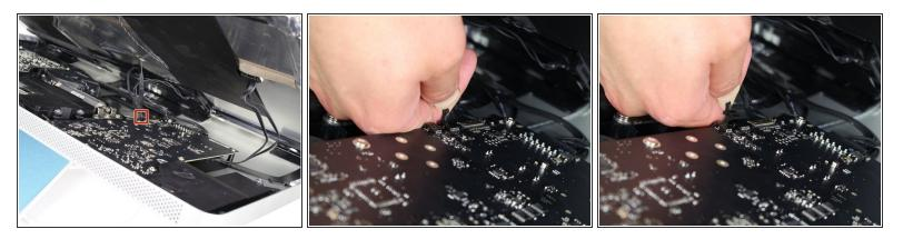
• For the first of the four wires (furthest away from the wire that is held in by a screw), grab onto the connector and pull slowly.
