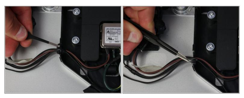
Next, remove the piece of electrical tape that is holding wires into the casing connecting to the power adapter.
