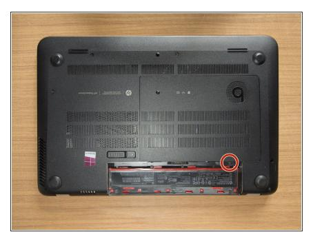
Remove the Phillips PM2.0×4.0 screw using a PH#00 screwdriver.
