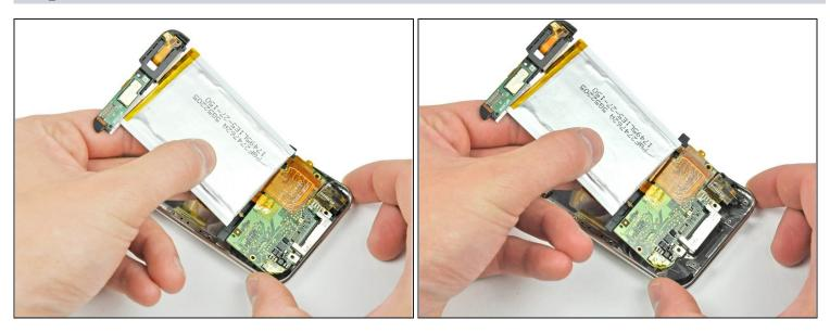
• Carefully lift the logic board assembly out of the rear case, minding any edges that may get caught.
