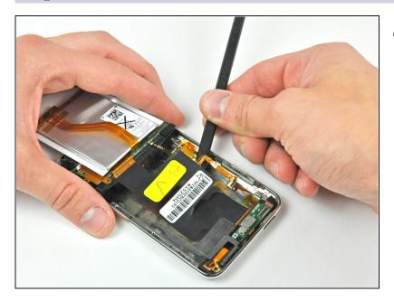
Insert the flat end of a spudger between the metal rear panel and Wi-Fi ribbon cable to further loosen the adhesive along the length of the cable.
