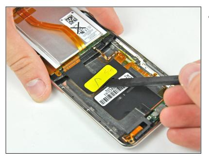
• Use the flat end of a spudger to separate the Wi-Fi ribbon cable from the adhesive securing it to the rear panel.
