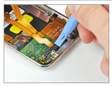
• Use an iPod opening tool to pry the display cable connector up off its socket on the logic board.
