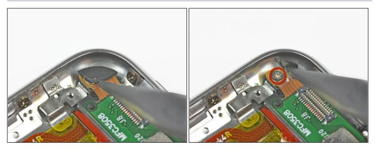
• Use the tip of a spudger to peel back the protective rubber grommet to reveal a hidden Phillips screw.
