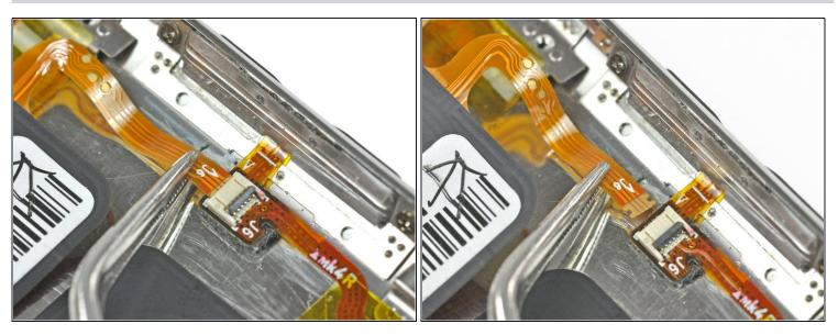
• Use a pair of tweezers to pull the control button ribbon cable straight out of its socket.
