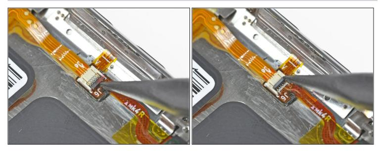
• Using the tip of a spudger, flip up the control button ribbon cable retaining flap.
