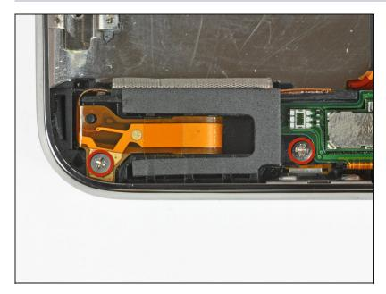
• Remove the two remaining Phillips screws securing the upper logic board to the rear panel.
