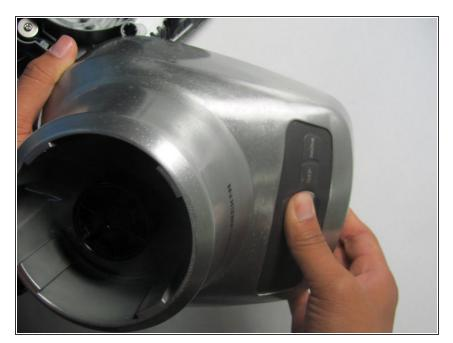
Push firmly from the outside of the blender on the face of the buttons to pop it out of its locked position.
