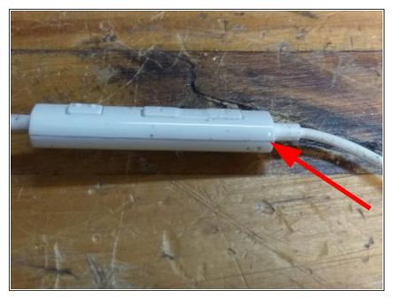
Find the edge of the control unit and get a very fine flathead screw driver (or a plastic pry tool which would do less damage)
