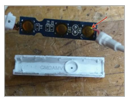
It is quickly seen that one of the wires has broken away from the circuit board (see image)
