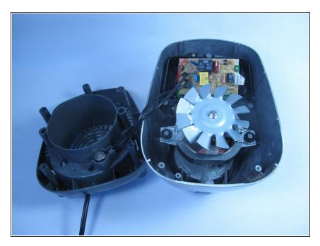
Lift the top half of the base from the bottom half of the base to reveal the internal mechanism.
