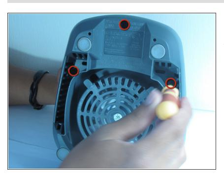
Remove the top three 1/4 inch base screws using a Philip's head screwdriver.
