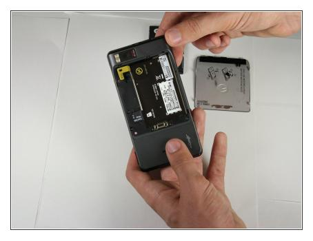
• The battery has been successfully removed.
