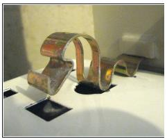
• Use prise tool to remove two case clips. Pull top of case towards you, rock case (almost whole cabinet: case top, front, left & right) on its bottom front edge as axis, lower front of case until it rests on floor.
