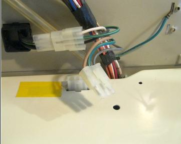
• Press on tab to release clip/latch. Grip connector, not wires, and pull it off of fixed connector.
