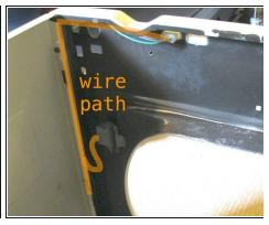
Case grounding wire is fastened on with one screw, 5/16 (five sixteenths) inch hexagon head.
