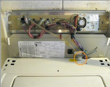
Control panel console is fastened with two screws. Remove screws, pull bottom end of control
