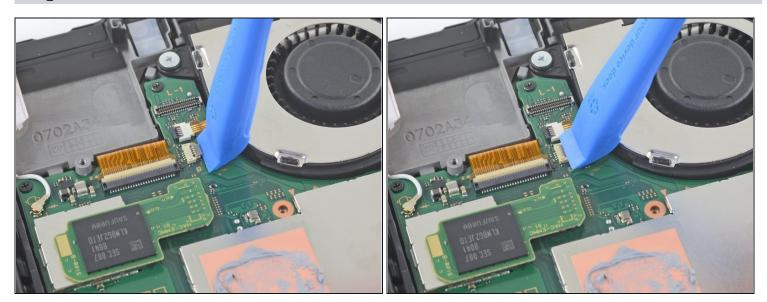
• Use an opening tool, spudger, or your fingernail to flip up the small, hinged locking flap on the fan cable <u>ZIF connector</u>.
