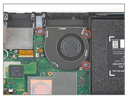
Use a JIS 000 screwdriver or an official iFixit PH 000 driver to remove the three 4.8 mm screws securing the fan.
