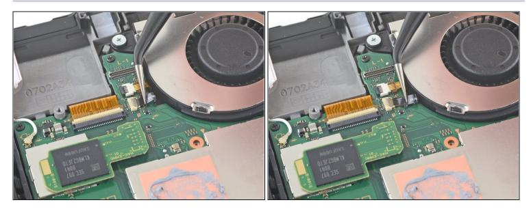
• Use a pair of <u>tweezers</u> to pull the fan cable straight out of its connector on the motherboard.
