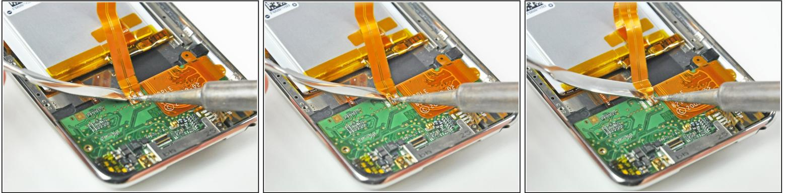
**i** The battery on the second generation Touch is attached via solder pads with small holes that go *through* the battery ribbon cable and attach to flat pads on the face of the logic board. In this step, you will heat each solder pad individually while using a metal spudger to pry it up from the logic board.
