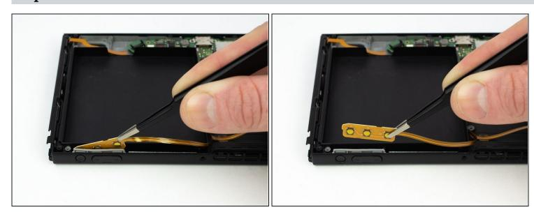
• Remove the power/volume board with a pair of blunt nose <u>tweezers</u>.
