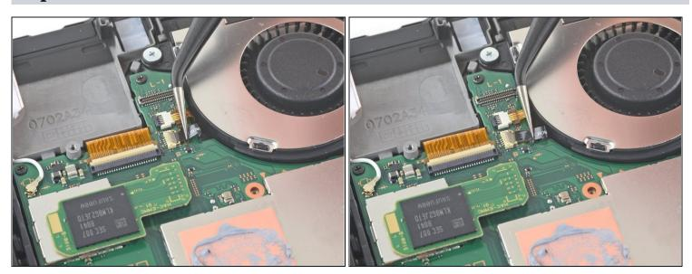
• Use a pair of <u>tweezers</u> to pull the fan cable straight out of its connector on the motherboard.
