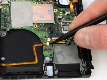
• Use a spudger to flip up the small black locking flap on the power/volume ribbon cable <u>ZIF</u> connector.
