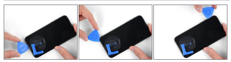
Slide the opening pick around the lower left corner and up the left edge of the iPhone, slicing through the adhesive holding the display in place.
