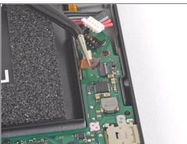
Use a pair of tweezers to slide the Joy Con rail data cable out of its connector on the motherboard.
