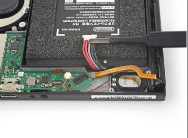
• Use your fingers or a pair of tweezers to lift the battery connector up and out of the way of the Joy Con rail's data cable.
