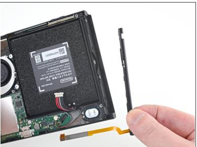
Remove the left Joy Con sensor rail from the device.
