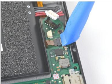
Use an opening tool, spudger, or your fingernail to flip up the small, hinged locking flap on the Joy Con rail data cable's <u>ZIF connector</u>.
