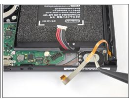
• Use your fingers or a pair of tweezers to lift the battery connector up and out of the way of the Joy Con rail's data cable.
