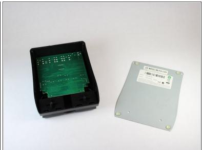
Remove the back panel to expose the motherboard.
