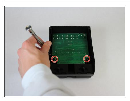
Remove the two 11mm #0 Phillips screws located at the bottom of the motherboard.
