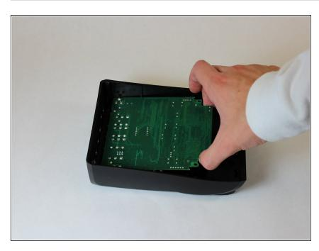
Lift the indented end of the motherboard opposite the input/output jacks. Then, pull away from the input/output jacks to slide the motherboard out of the casing.
