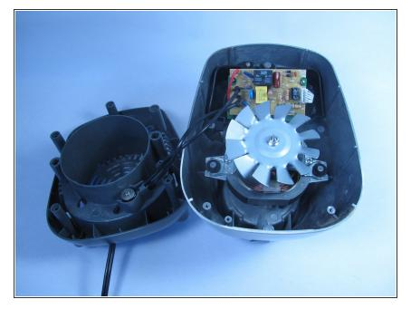
• Lift the top half of the base from the bottom half of the base to reveal the internal mechanism.
