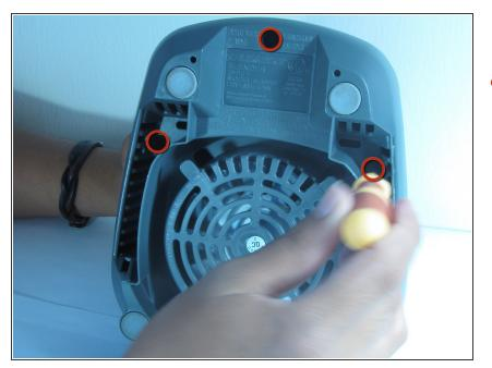
Remove the top three 1/4 inch base screws using a Philip's head screwdriver.
