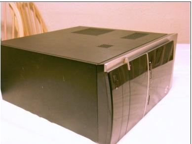
Lay the tower down carefully on its right side, with the vents pointing up.
