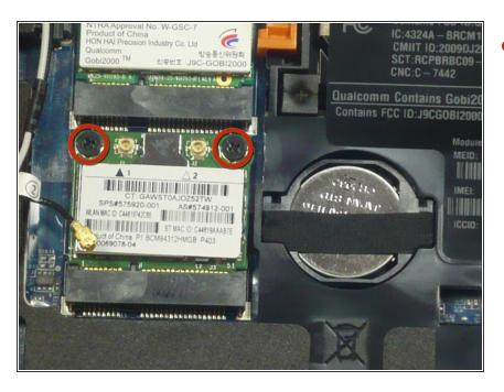
Remove the two 3.9 mm screws on top of the WiFi card using the Phillips #00 screwdriver.
