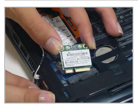
Gently pull the WiFi card out of its slot. Be sure to pull the card up and out of the slot towards you.
