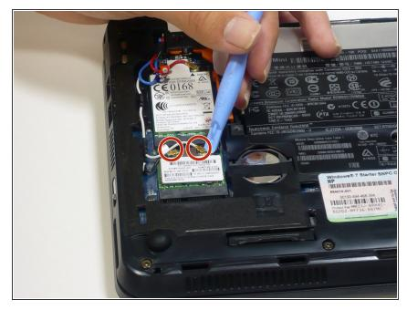
Pop out the two gold connectors from the antenna wires on top of the WiFi card using a plastic opening tool. This will allow you to dislodge the WiFi card from the rest of the netbook.
