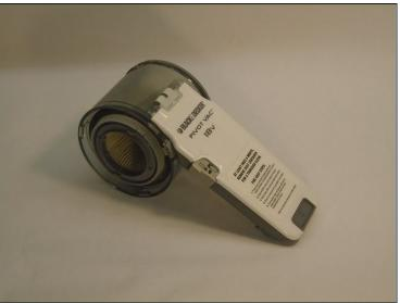
• To take off the nozzle, filter, and catch bowl first start off by pushing in the button identified with a red square and twist that part of the device toward the handle portion of the vacuum and it should click and pop off the chassis.
