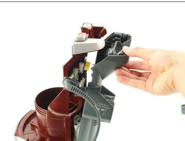
Use the metal spudger to pry off the back panel.
