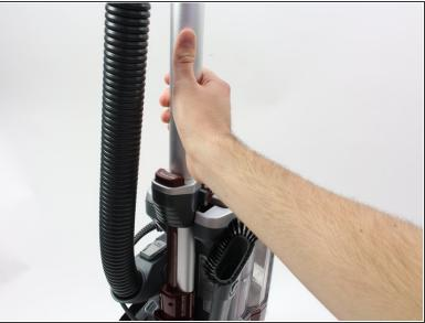
Press the Wand Release button and pull up on the metal tube to remove the entire hose.
