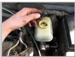
Use caution while handling brake fluid. Brake fluid strips paint and dissolves plastic.
