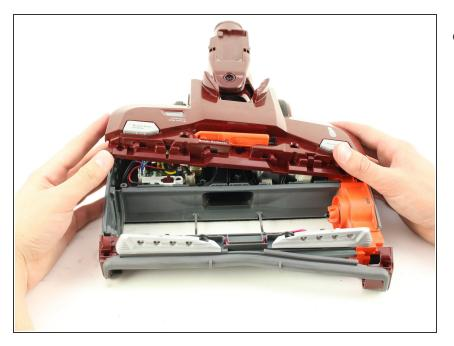
Remove the red cover by lifting upward.
