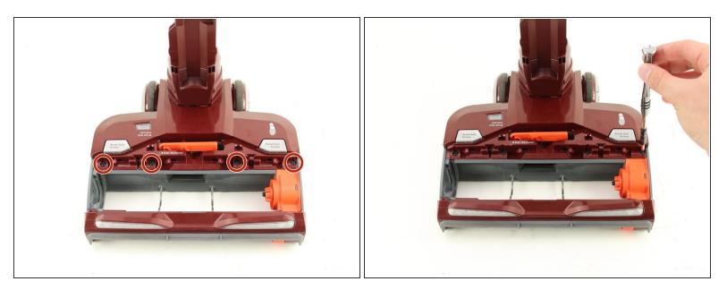
Use the T20 screwdriver to remove the four 17 mm screws by turning counterclockwise.
