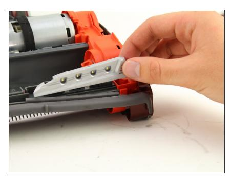
• Remove the light fixture by lifting it up.
